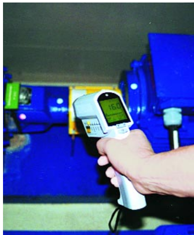
Motor Bearings Check for worn bearings before they fail.
