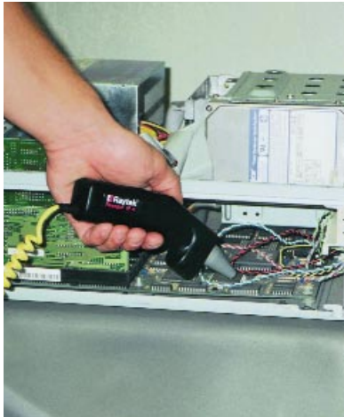
Small Circuits Isolate short circuits and bad connections.
