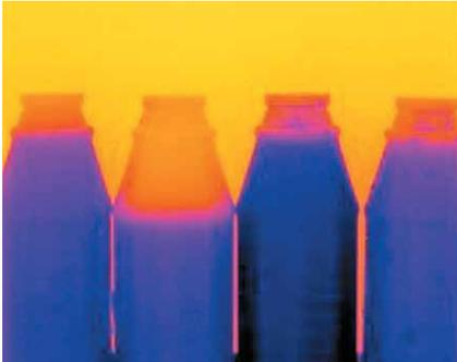
Detecting liquid levels in visually opaque bottles.
